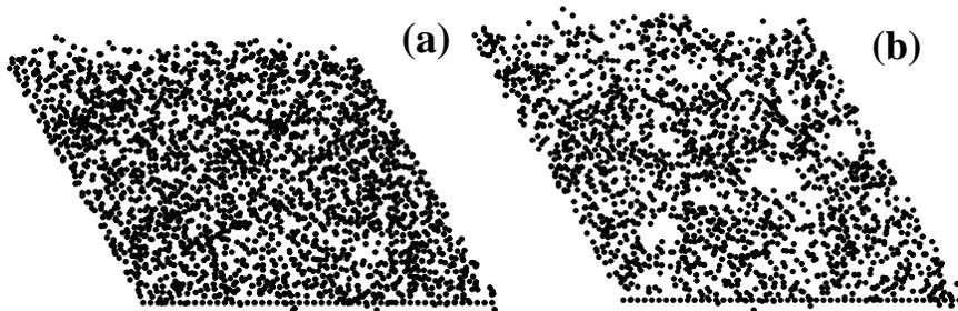
**Fig. 1.** Bulk configurations of a  $48 \times 48$  system, shown after relaxation. The nodes, which represent crosslinkers, are shown as dots. For clarity the bonds, which represent polymer chains, are not shown. The inhomogeneity of the crosslinker distribution in the bulk is visible. (a) Without holes. (b) With 18% vacant nodes. Even for this small system the different roughness of the surfaces is apparent to the eye
